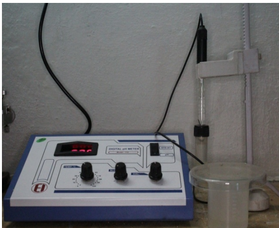
Figure 1: DIGITAL PH METER
