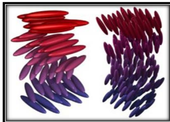
Figure 6: Schematic of ordering in chiral liquid crystal phases.
