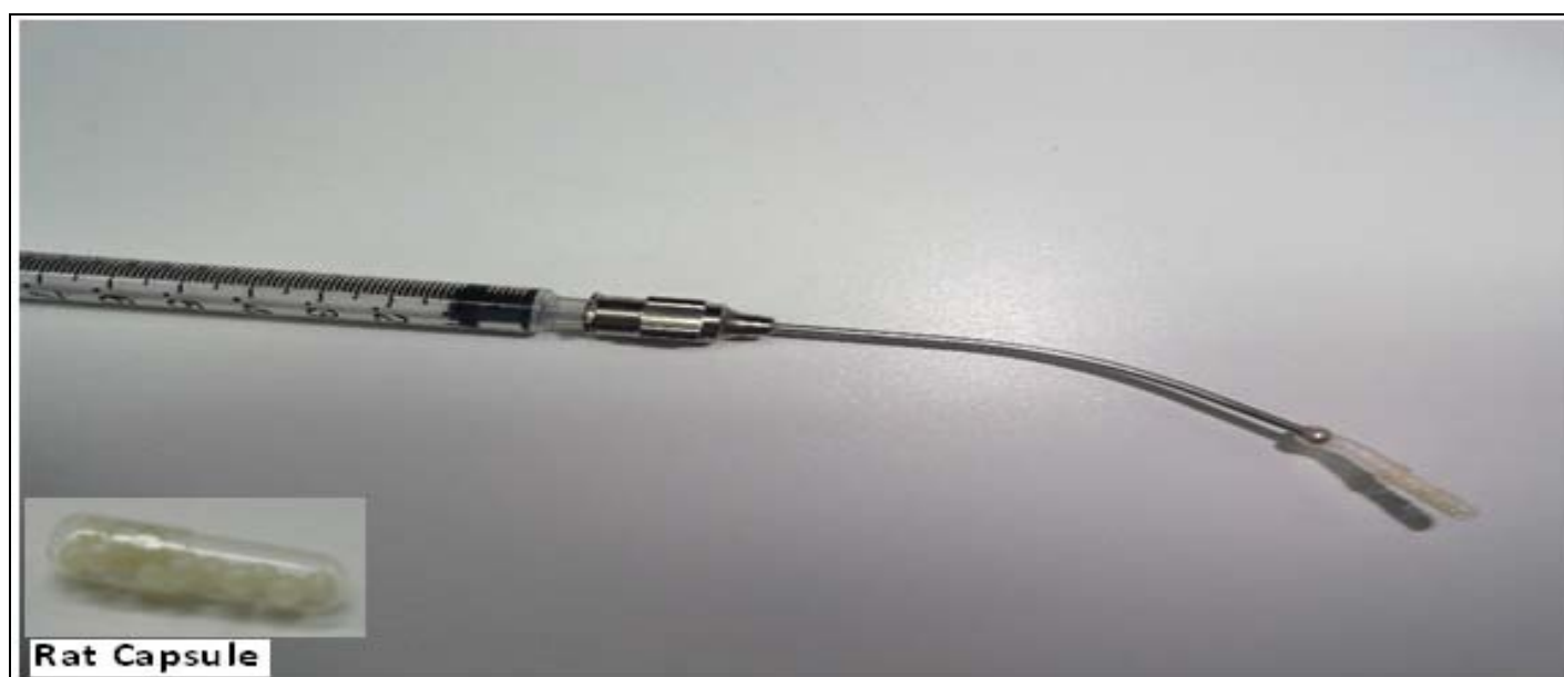
Figure No.2: A special devices designed for oral administration of enteric coated pellets to rats.
