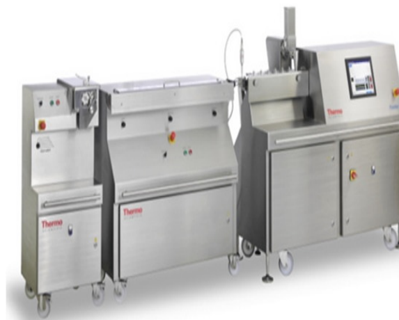
Figure 2: Hot melt twin screw extruder (Image courtesy of Thermo Fisher Scientific Inc.)
