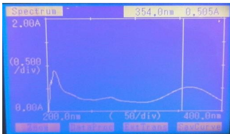
Figure 2: UV scan of Meloxicam in Phosphate buffer (pH 7.4) at \lambda max at 354 nm
