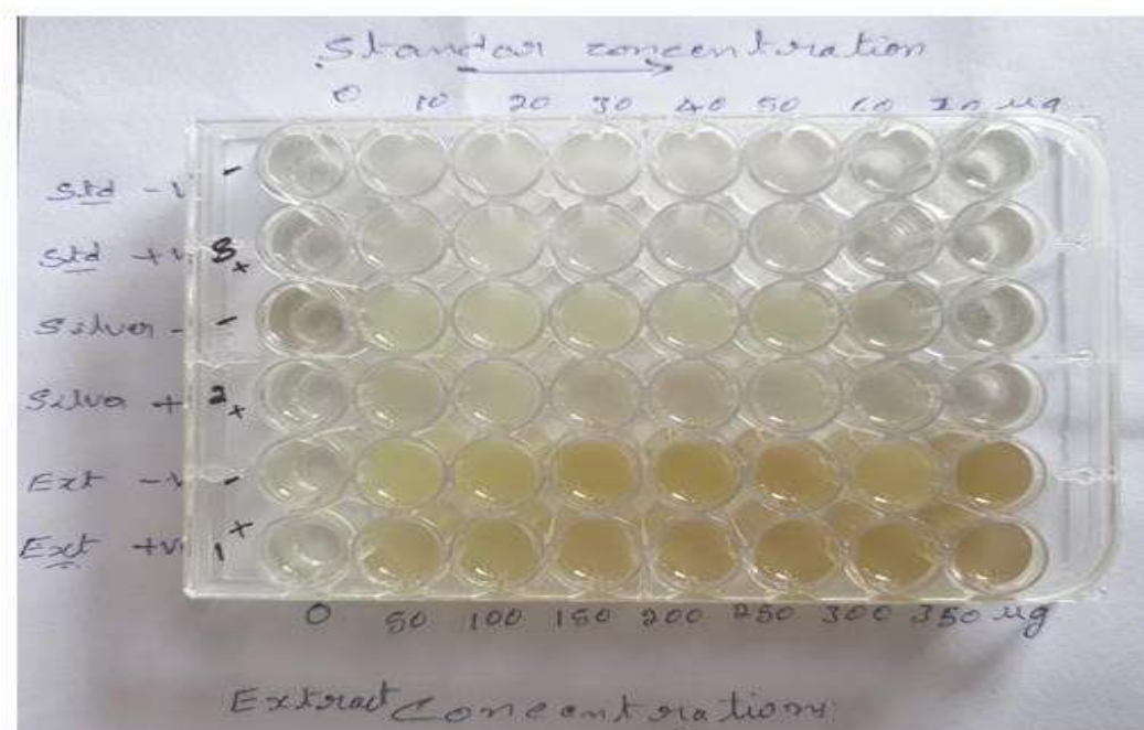
Figure 22: MIC of Albizia amara AgNPs, Albizia amara extract, standard Std. kanamycin against bacterial strains
