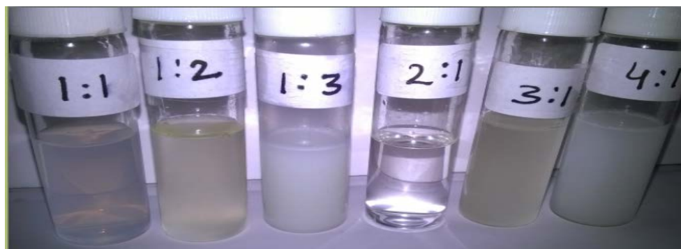
Figure 1: Visual observations of transparent and easily flowable o/w nanoemulsions made by different oil and Smix ratio
