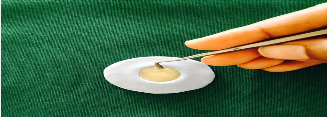
Figure 1: Composite disks being made with a mould of putty consistency rubber base material
